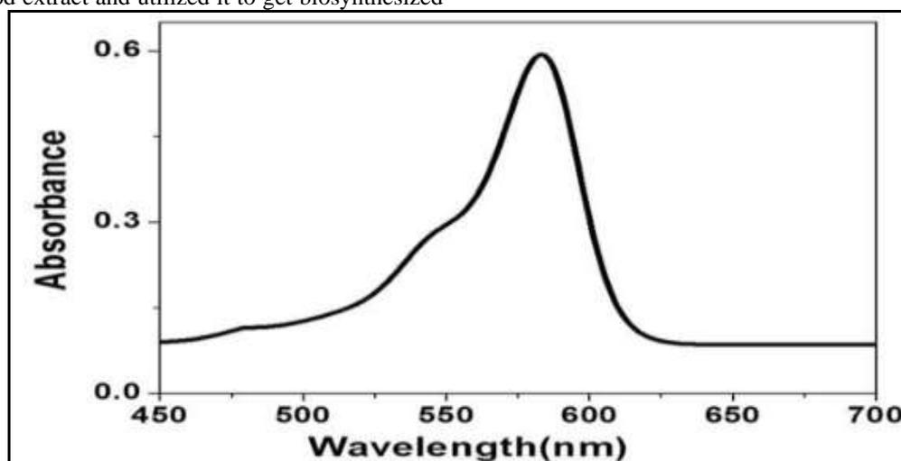
**Figure 1.** Ultraviolet visible Spectra of copper nanoparticles biosynthesized by water caltrop extract treated with  $0.1 \text{ mgL}^{-1} \text{ CuSO}_4 \cdot 5\text{H}_2\text{O}$  using hot plate with magnetic stirrer. Graph plotted Absorbance ranges 0 to 0.6 vs wavelength ranges 450 to 700 nm. Maximum absorbance was 0.6 at 560 nanometer (nm) wavelength.
