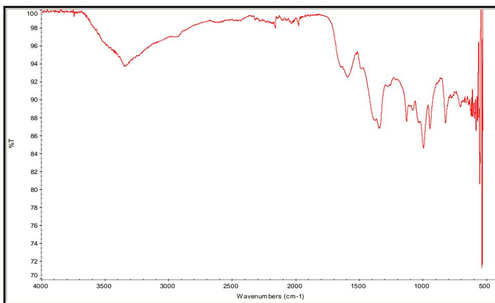
**Figure 2.** FT-IR spectra determines the molecular structure of water caltrop pod (WCP). Graph plotted Transmittance percentage (% T) vs wavelength ranges from 500 to 4000 per centimeter ( $\text{cm}^{-1}$ ). Peaks appeared were  $3341.09$ ,  $1594.86$ ,  $1340.08$ ,  $1129.96$  and  $945.23 \text{ cm}^{-1}$ .
