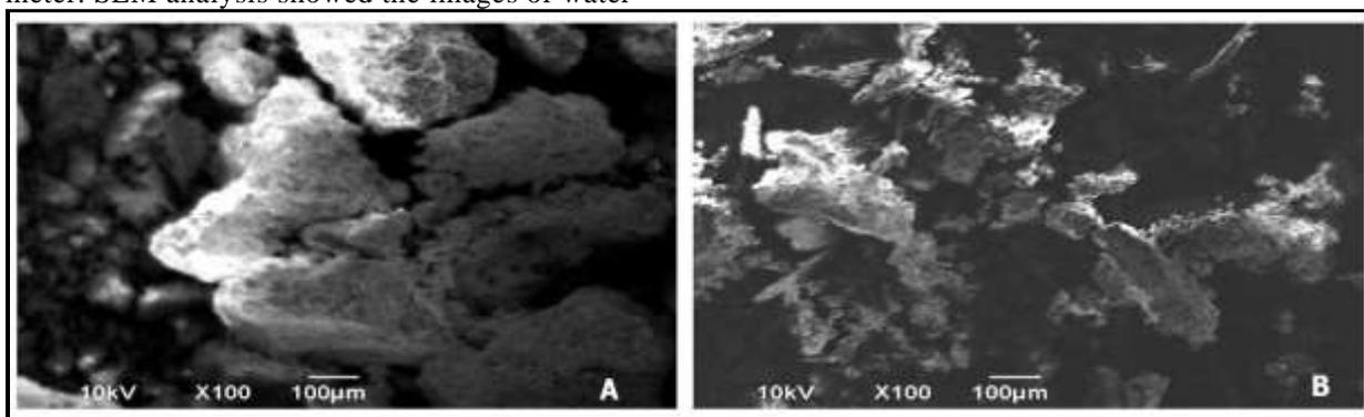
**Figure 3.** (A) and (B) scanning electron microscope (SEM) image of water caltrop pod and copper nanoparticles respectively. The surface morphology of water caltrop pod and copper nanoparticles was elaborated by Hitachi S-2300 SEM with 10 kV at x100 resolution and 100 micro meter ( $\mu\text{m}$ ). The SEM was equipped with EDX, which elaborated the elemental composition of WCP and CuNPs surfaces. The samples were carbon-coated using Edwards-Scan coat.
