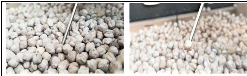
Figure 4. Temperature recording and seed moisture at different depths using pointed sensor needle.
